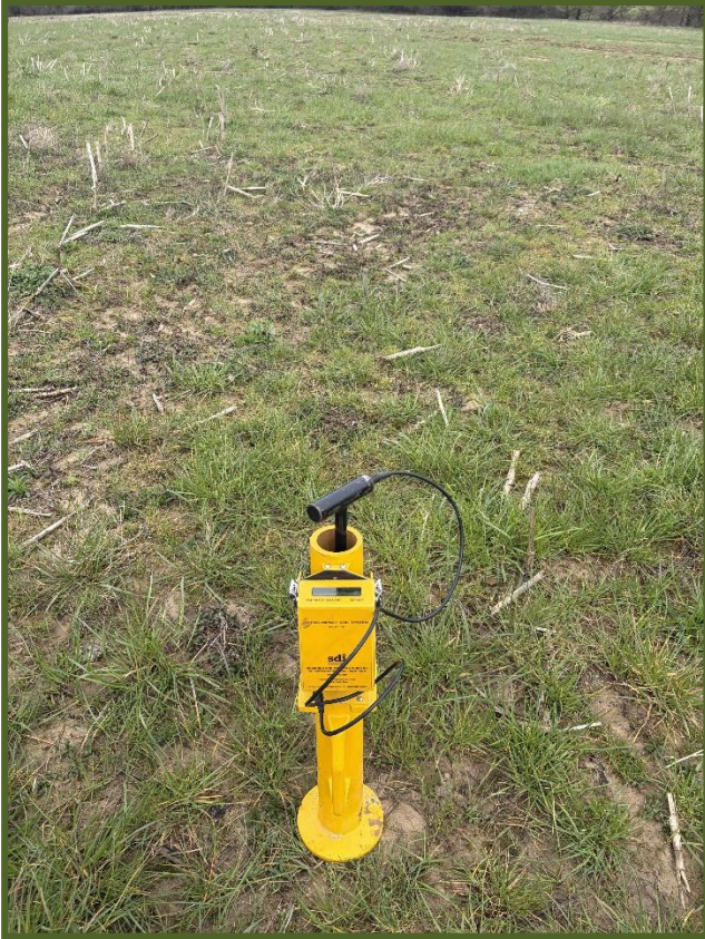
Plate 18 – Surface harness testing with 2.25kg Clegg Hammer
