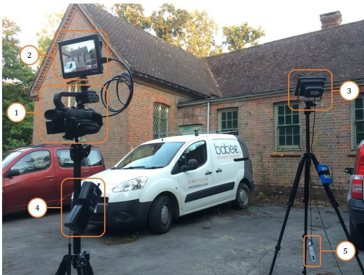
Photo 1. (1) Canon XA series video camera, (2) 7" high-definition screen attached to NVA (used at attended survey locations only), (3) Infrared floodlamp, (4) Batlogger-M, (5) Thermometer.
