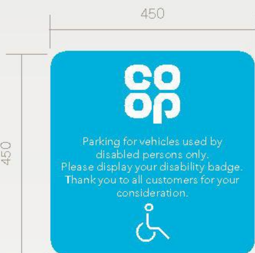
Item 6 1No 3mm ACM with applied vinyl and anti-graffiti laminate. Size: 450x450mm Scale: 1:10
