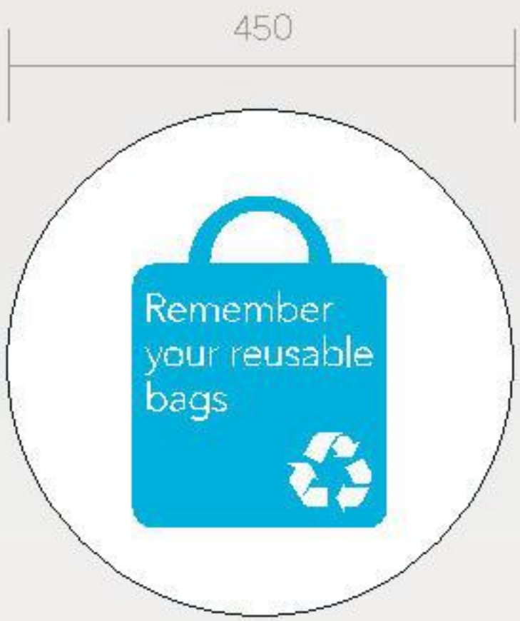
Item 9 1No 3mm ACM with applied vinyl and anti-graffiti laminate. Size: 450x450mm Scale: 1:10
