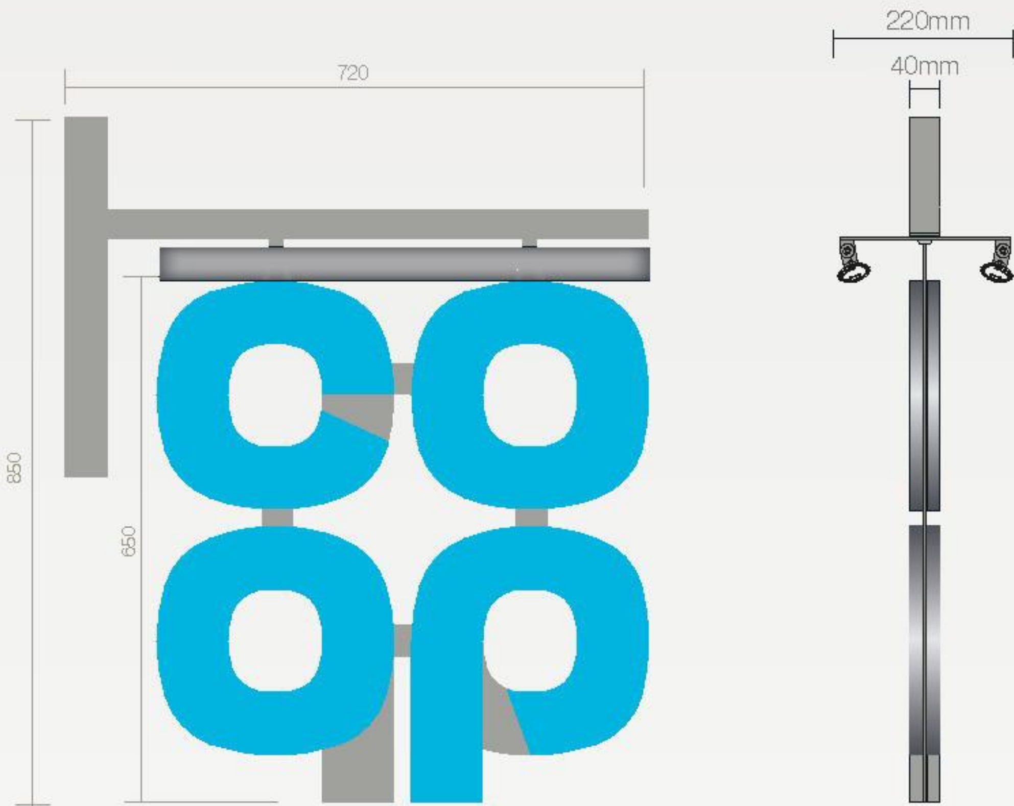
Item 3 Externally illuminated by LED trough light projection sign Size: 720x850mm Scale: 1:10
