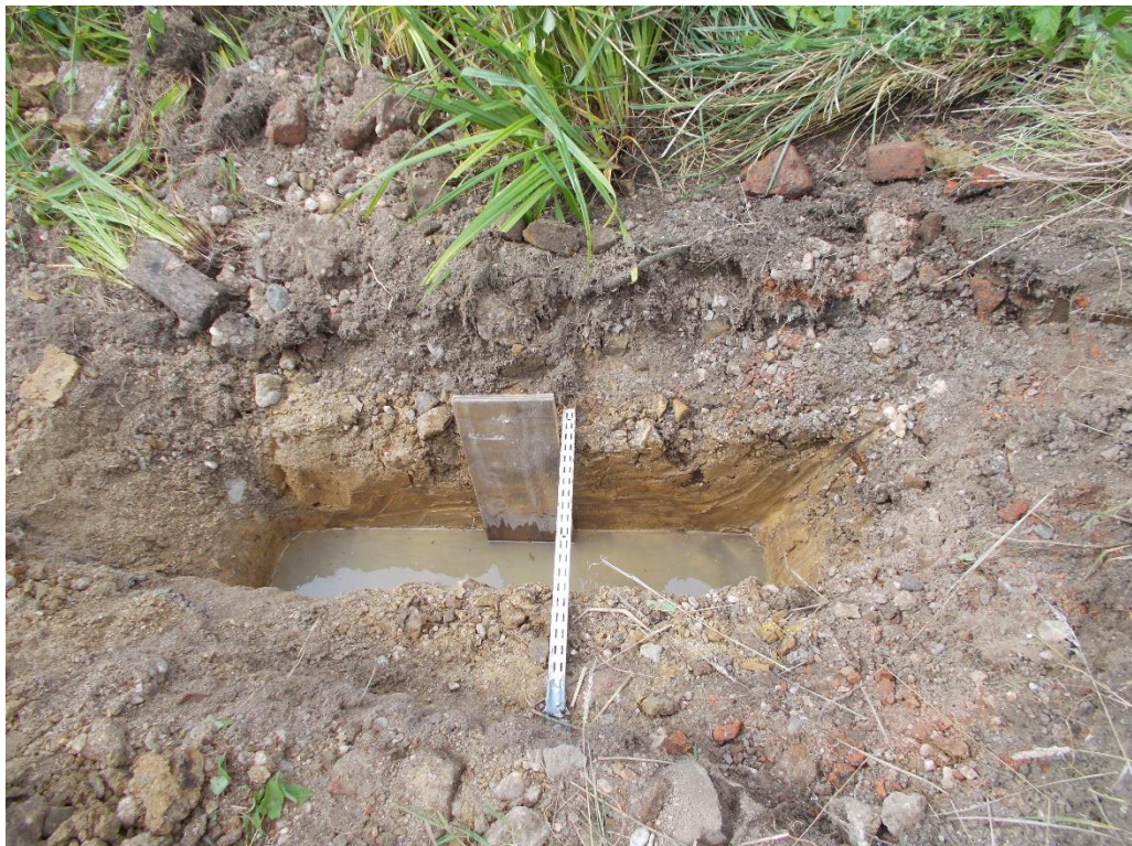
Photo 6: Percolation Test Pit PTP 2.
