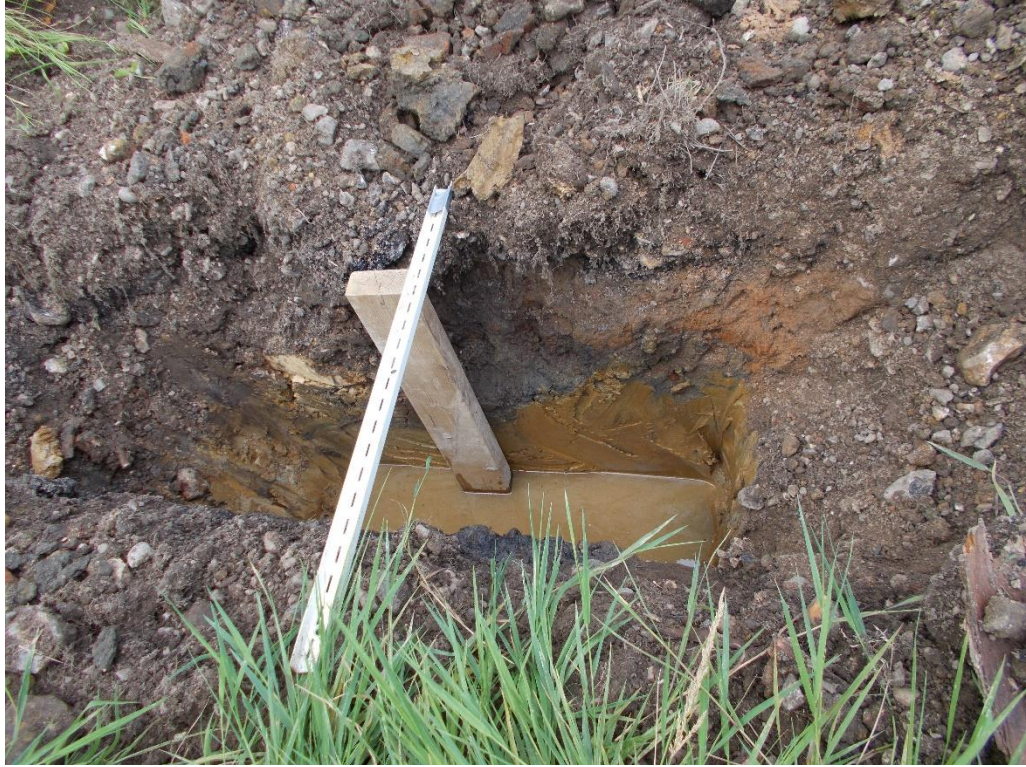
Photo 5: Percolation Test Pit PTP 1.
