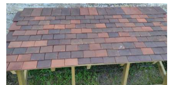
Image of proposed Spicer handmade peg tiles (Hanbury range). Sample panel laid in even mix of the following colours: Antique Dark, Antique Medium and Antique Red. Note sample panel previously proposed on The Mansion roofing project.
