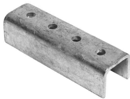
3. Galvanised pre-drilled channel (F.H. Brundle, PCB146/41, product code 50CF3341), 132 x 44mm.
