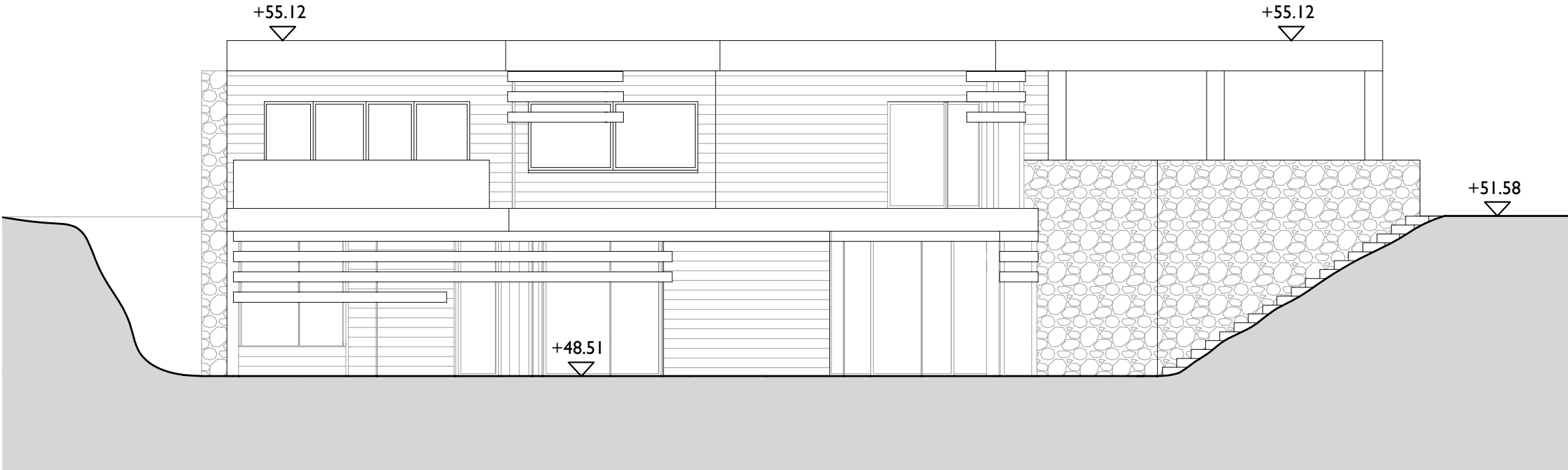
+EL Proposed south elevation - scale 1:100 at A3 Scale in Metres 0 1 2 3 4 5
