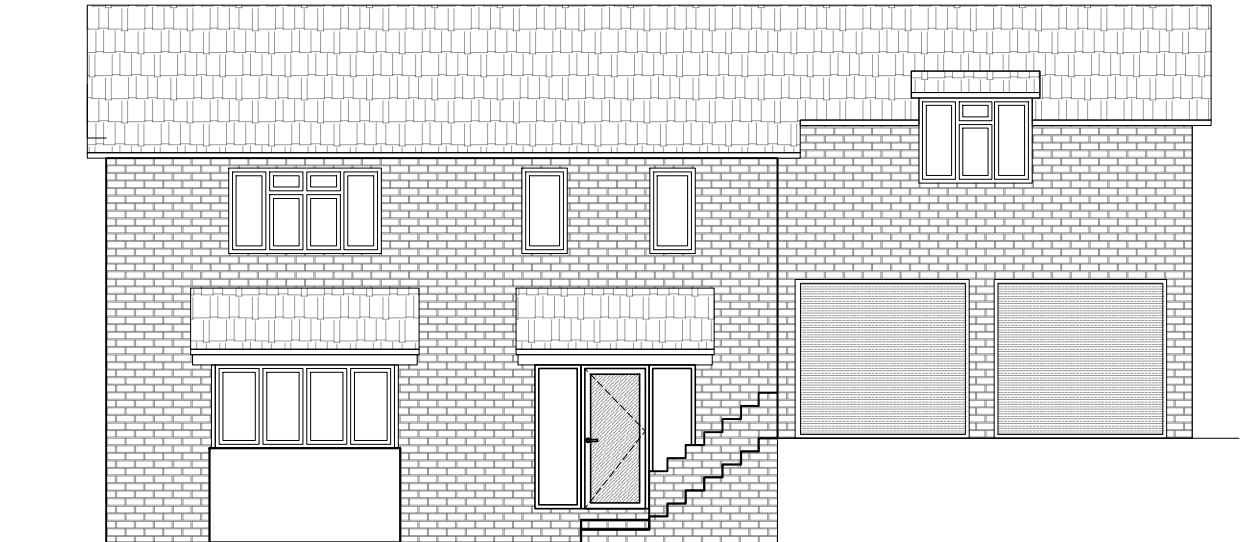
EXISTING FRONT ELEVATION
