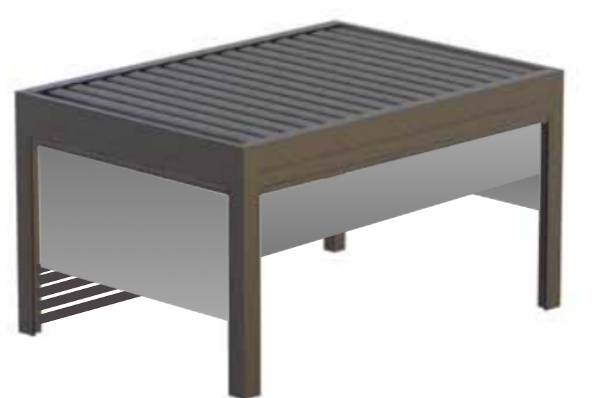
Isometric projection (Not to Scale) (Showing louvres to rear, and mesh blinds to front and sides, pulled down to varying degrees)
