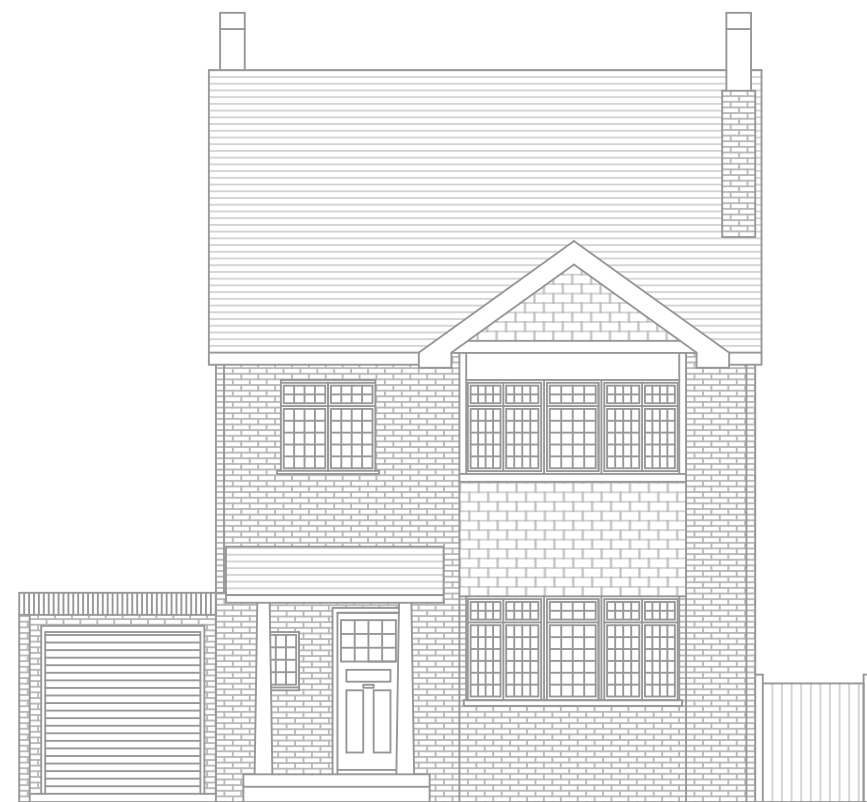
Existing Front Elevation (NW) Scale 1:100
