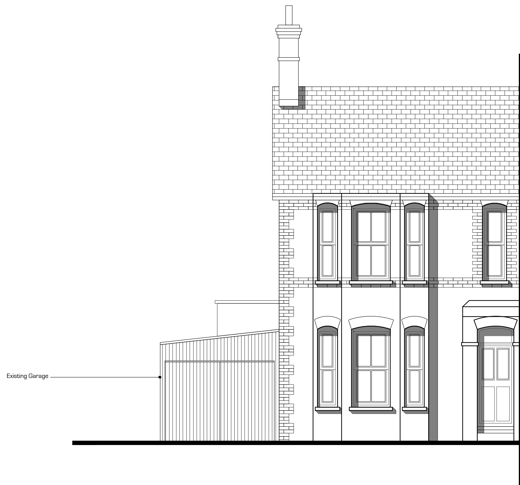
01 Existing Front (East) Elevation 1:50@A1
