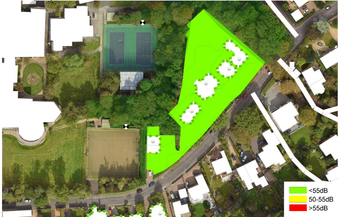
Figure 5.2: Estimated average noise levels ( L_{Aeq,1hr} , dB) at the nearest noise sensitive receptor and in external amenity areas due to road traffic noise
