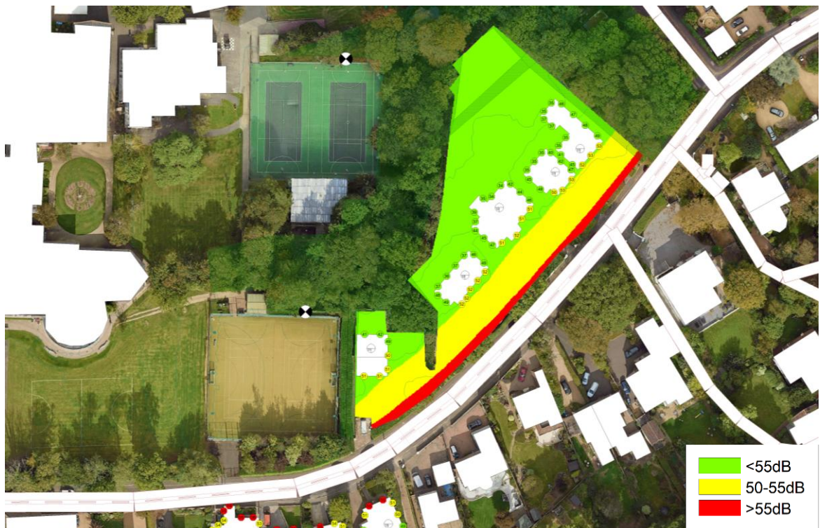
Figure 5.2: Estimated average noise levels ( L_{Aeq,1hr} , dB) at the nearest noise sensitive receptor and in external amenity areas due to road traffic noise
