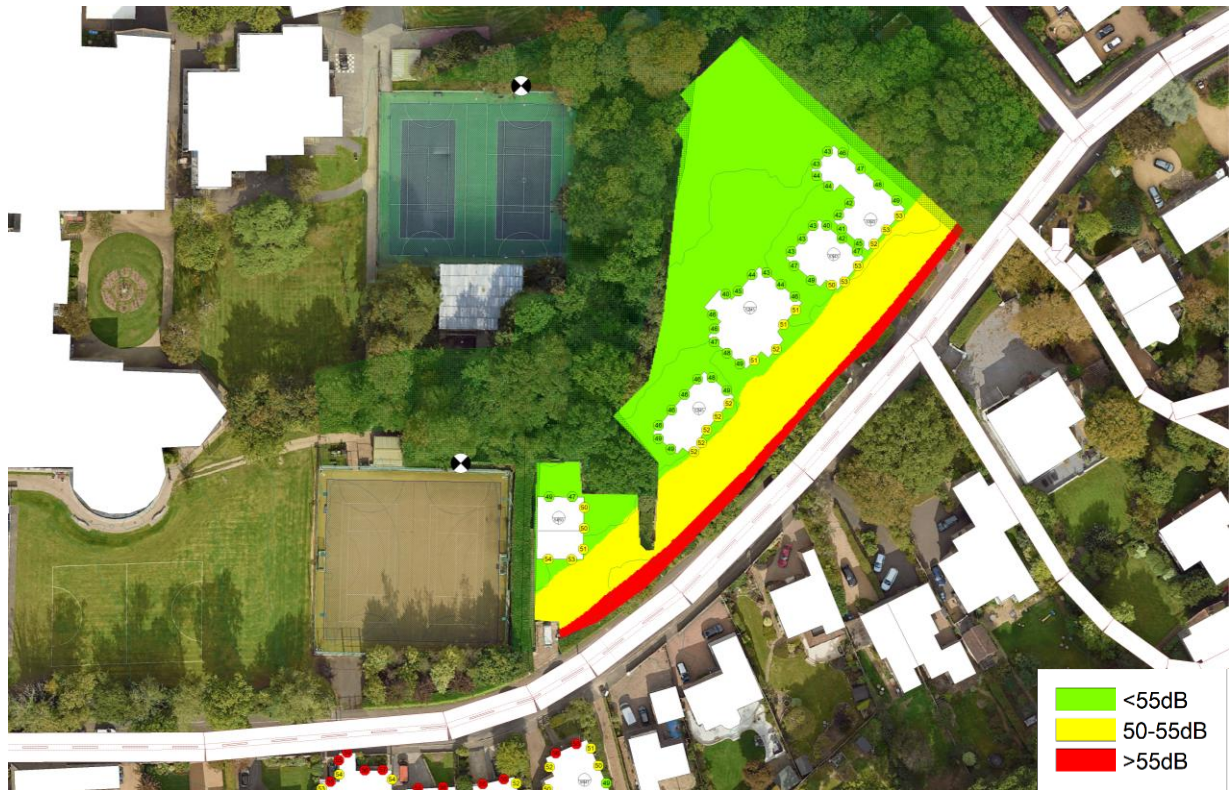
Figure 5.3: Estimated average noise levels ( L_{Aeq,1hr} dB) at the nearest noise sensitive receptor and in external amenity areas: road traffic noise and both sports pitches in simultaneous use
