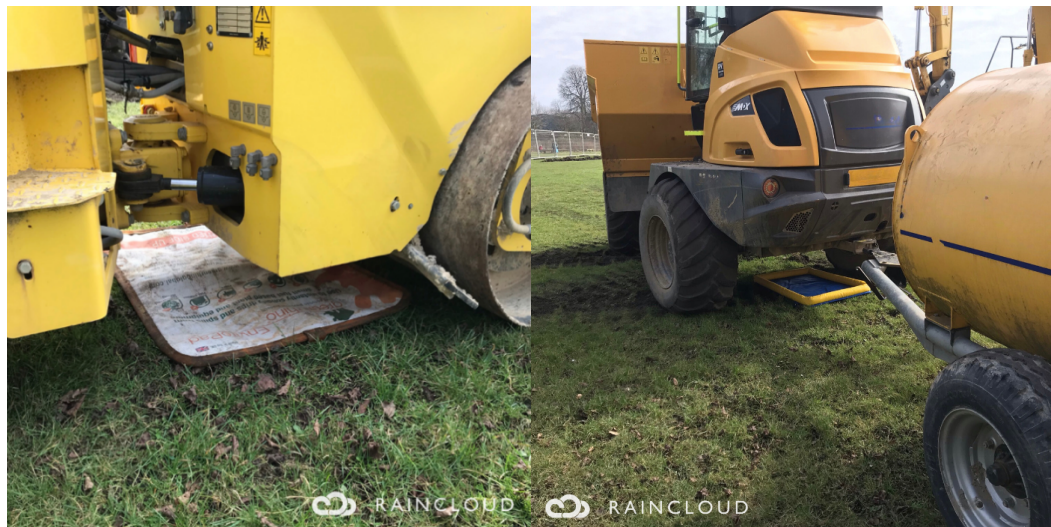
Figure 5: Drip trays and pads to limit uncontained chemical spillages
