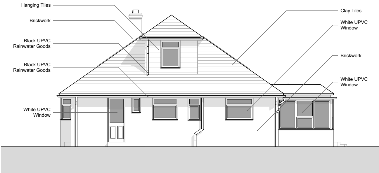
Existing North Elevation
