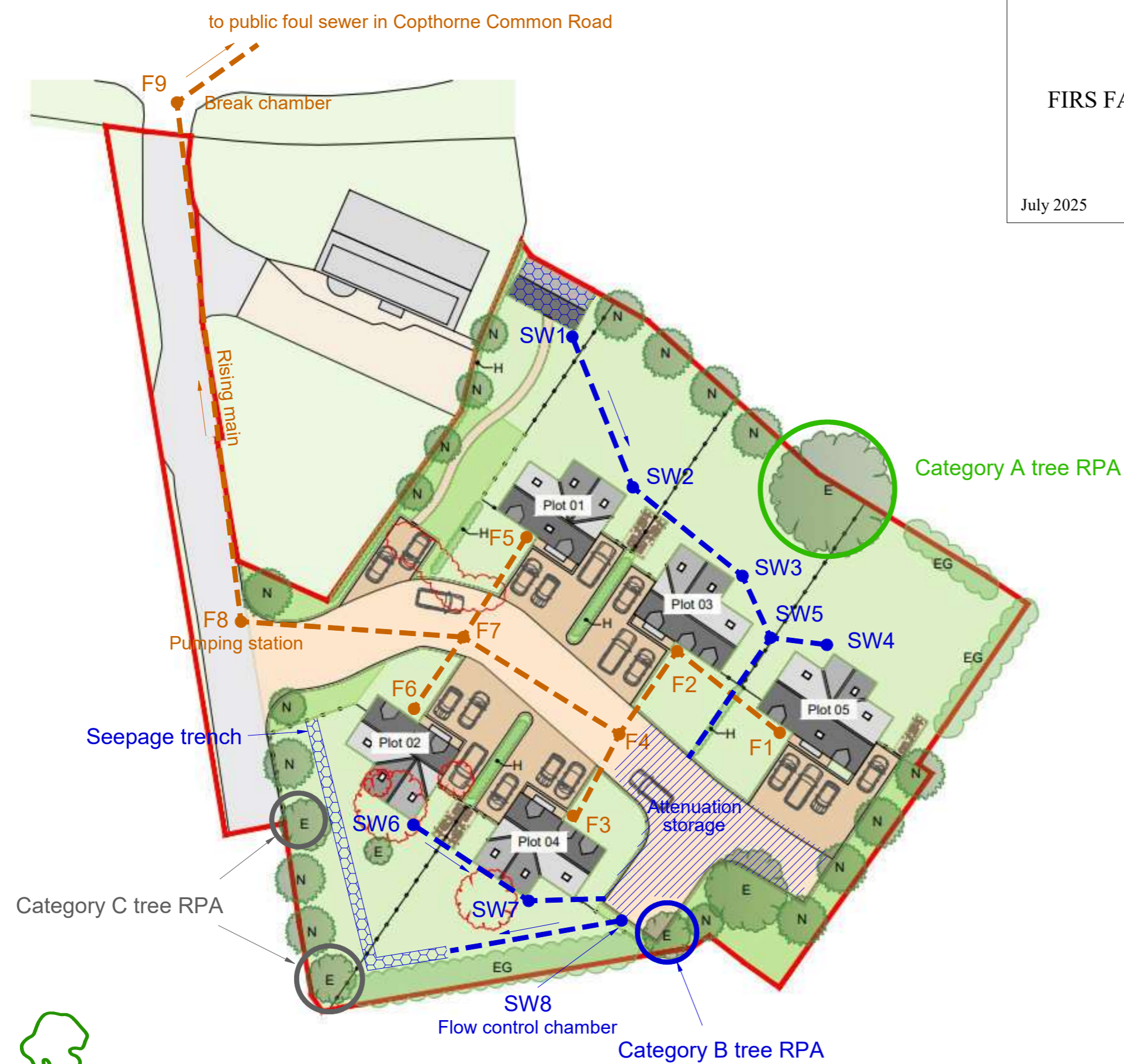
Figure 4: Suggested Drainage Arrangement
