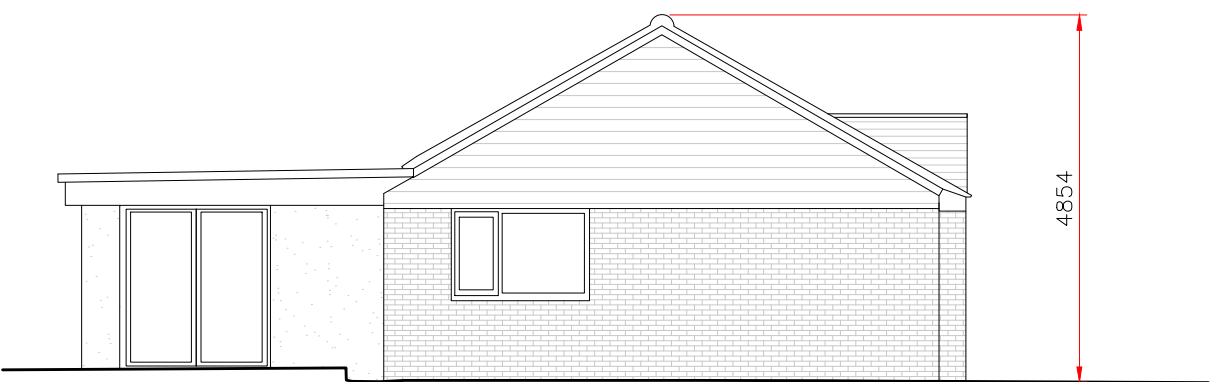
PROPOSED SIDE ELEVATION (SW) 1:100
