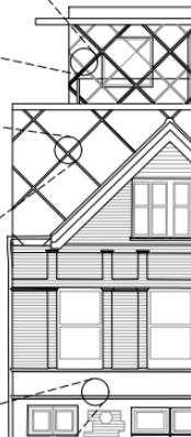
Vertical metal cladding to cores The proposed cores have a vertical standing seam, to differentiate them from the existing building, since these are a new building element
