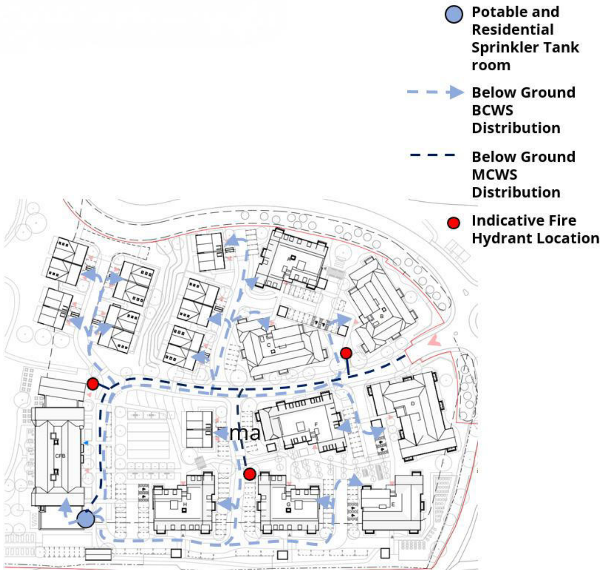
Figure 3 - Site Water Distribution
