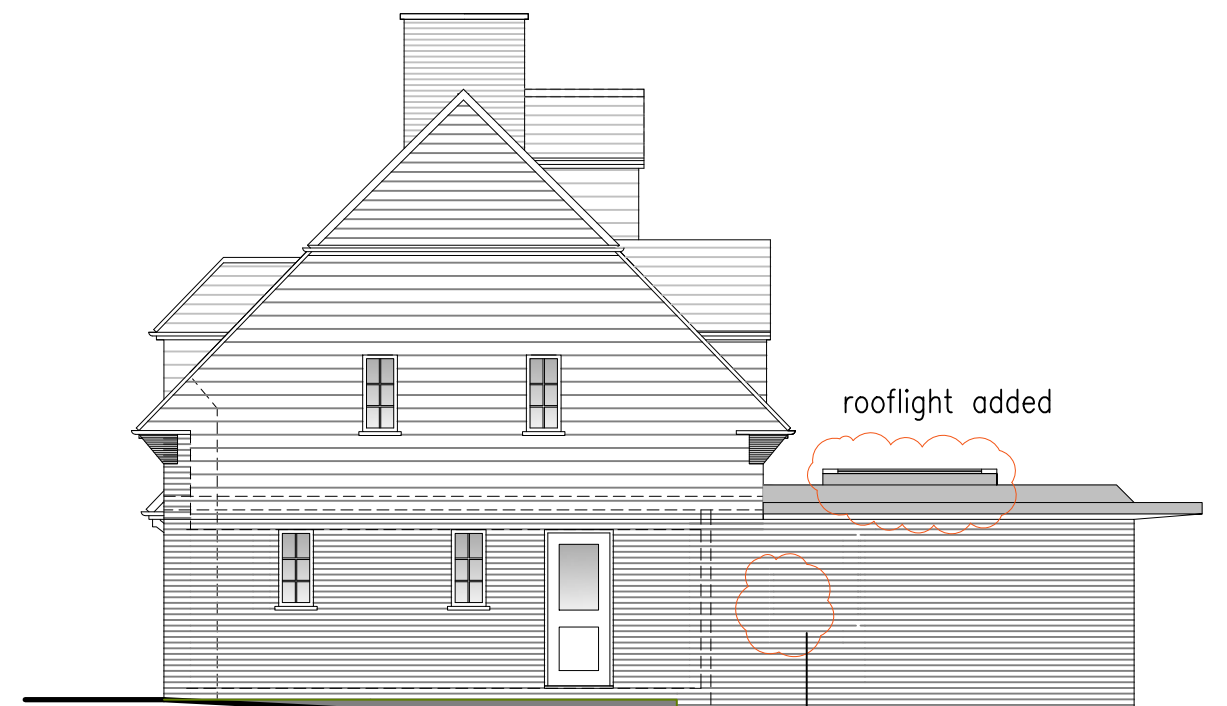
Side Elevation (South-East) 1:100
