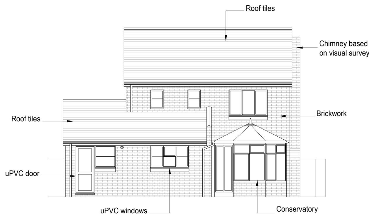
Existing Rear Elevation 1:100
