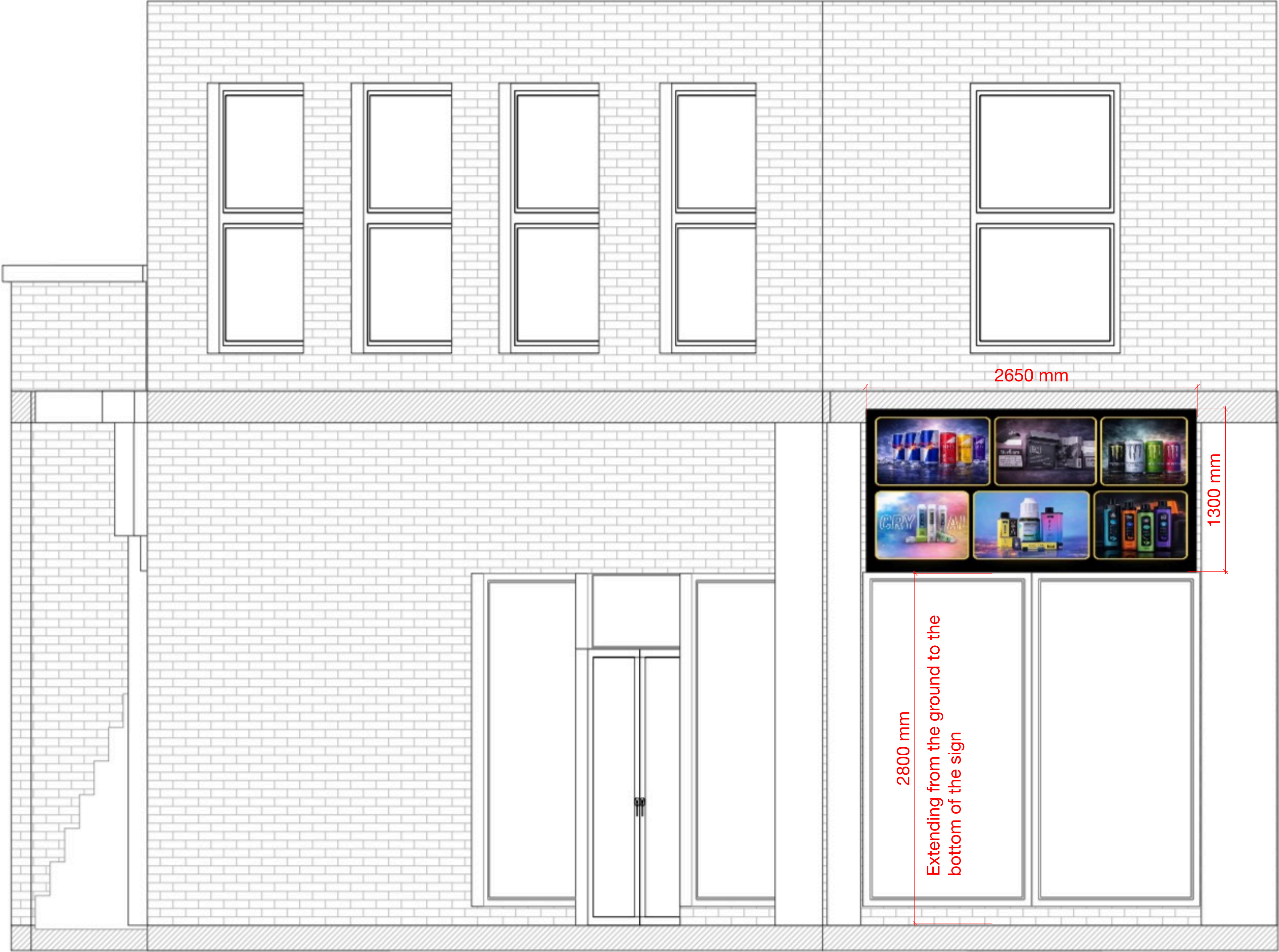
Proposed Front Elevation - Top Store Grocery (Left-hand side non illuminated vinyl poster signs) Scale: 1:20
