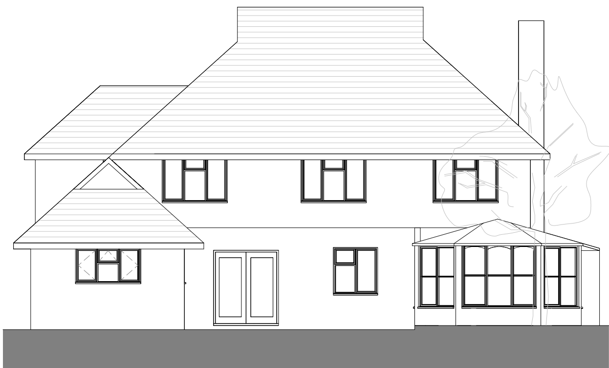
South Elevation as Existing 1 : 100
