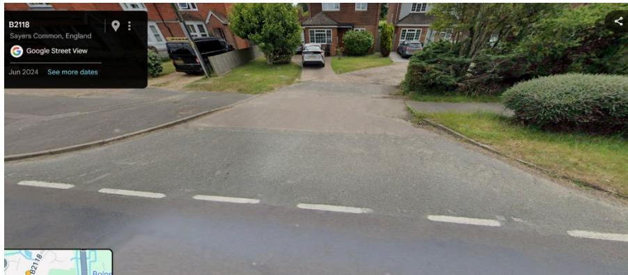
Tactile paving should be provided on the footway at the northern access (Roundhay). Kerbs will require adjustment to accommodate the tactile paving and footway may require reconstruction.
