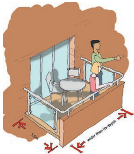
Figure 10.6: Potential dimensions for balconies.
