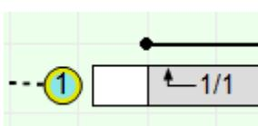
A Lane showing a yellow and blue Lane number circle is a signalled Lane which also gives way to other traffic. They are typically used for right turning lanes within a signal junction although they may also be used in more specialised situations such as signal & give-way left slips.
