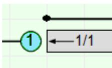
A Lane showing a blue Lane number circle is an unsignalled Lane which gives way to other traffic. They are typically used for minor arms of priority junctions and unsignalled left slips within signal junctions.
