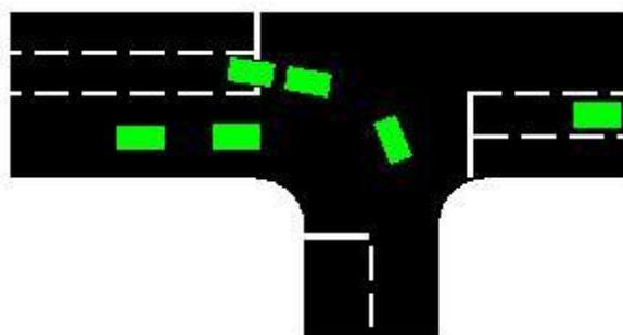
LinSig uses the give way model described above to model the capacity of the right turn during the period it is opposed by oncoming traffic. Common practice in the UK for many years has been to use Tanners formula to calculate the amount of traffic turning in gaps. This can be closely approximated in LinSig 3 by using 1440 for Intercept and 1.09 for slope in the give way model.
