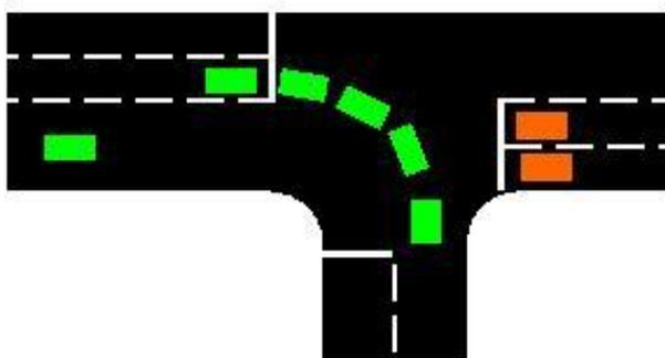
The Capacity during the time when the right turn is unopposed, possibly whilst an Indicative Green Arrow is running, is calculated using the value of 'Saturation Flow when Unopposed' defined for the give way Lane. This may be lower than the Lane's Saturation flow if the right turners share the Lane with Ahead traffic as the Lane's Saturation Flow relates to the Ahead movement.
