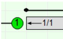
A Lane showing a green Lane number circle is an unsignalled Lane which does not give way to other traffic. They are typically used for through traffic on major roads at priority junctions and exit Lanes. This type of Lane is sometimes referred to as a 'bottleneck'. Unsignalled Lanes can either be unconstrained with effectively an infinite saturation flow or a saturation flow can be specified.
