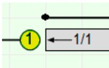
A Lane showing a yellow Lane number circle is a standard signal controlled Lane which does not give way to other traffic.
