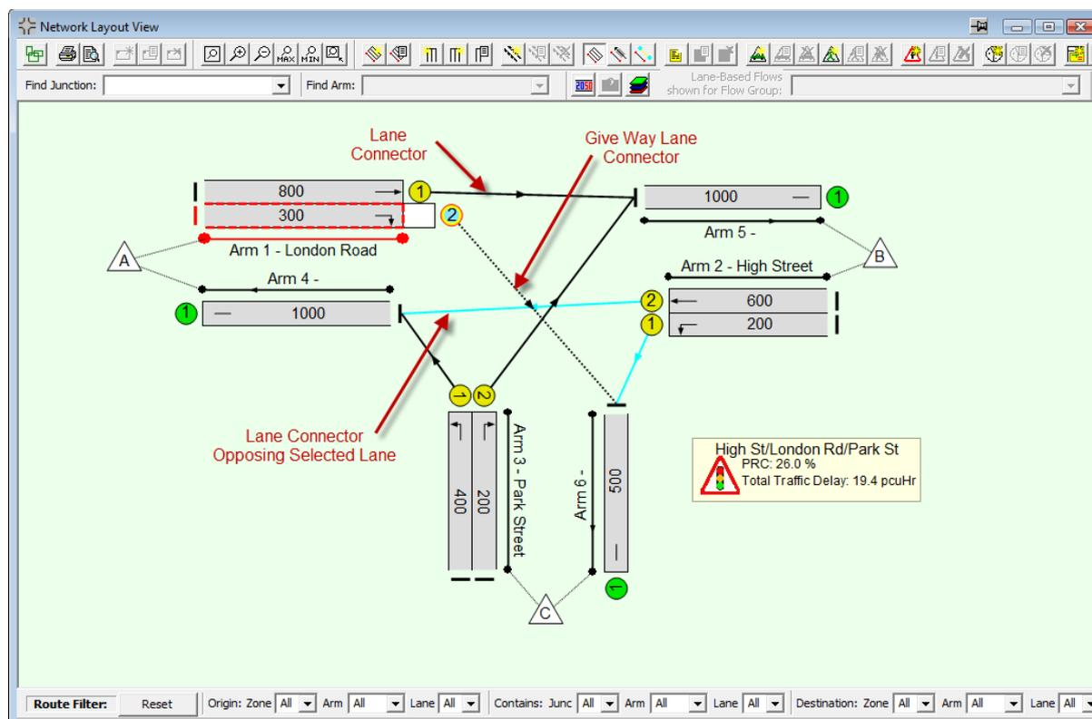
The diagram above shows Lane Connectors joining Lanes to other Lanes. Lane Connectors representing traffic movements which give way to other Lanes are shown dashed. If a give-way Lane or give-way Lane Connector is selected with the mouse its opposing Lane Connectors are shown highlighted.
