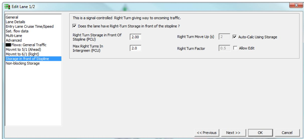
Lanes which include Right Turns that have Storage in front of the Stop Line require additional settings to model all the components of right turn capacity modelled by LinSig. These settings are contained on the 'Storage in Front of Stop Line' tab. They include:
